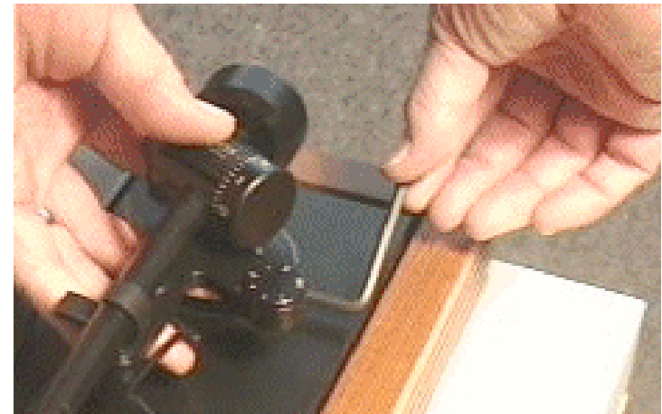
8. Supporting the Tonearm as shown loosen the grub screw with 4 mm Allen (hex) key and remove from turntable. With the Ittok LVII, first un-clip from the arm rest and, supporting as shown, lift clear of the turntable.
